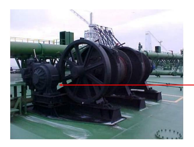
Hydraulic Motor, The driving Power for the winch
