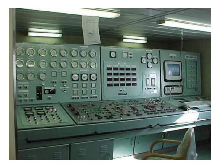
Pumps and Valve operations for Cargo And Ballast are controlled from CCR
