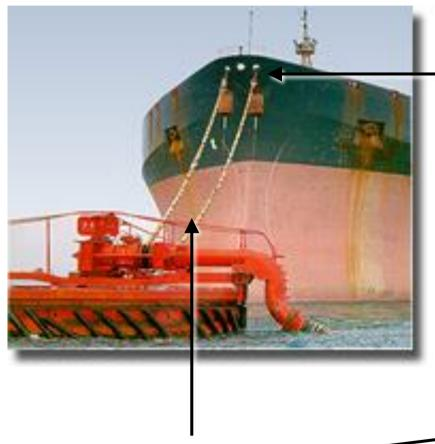
SBM chain made fast to the ship
