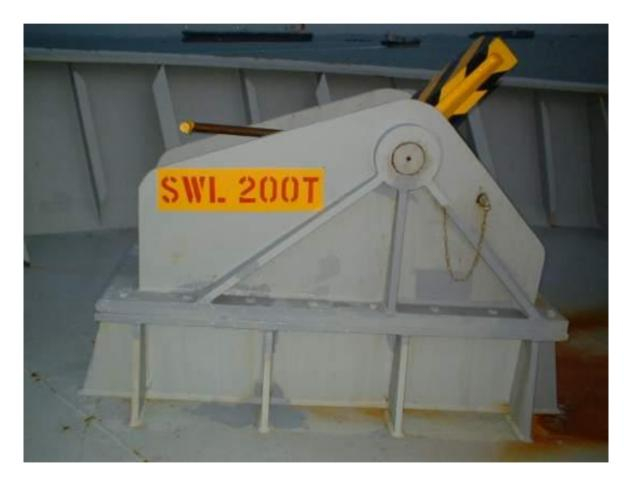
The Chain Stopper is installed on the Foc'sle deck
