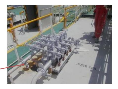
Steam (Example) runs through these coils which in turn heats up the cargo in the tank
