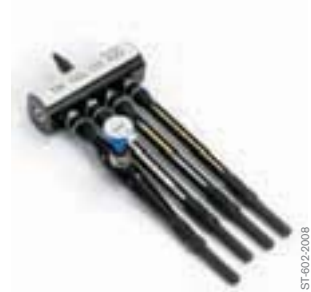
Impactor with Adapter in Aerotest Simultan
