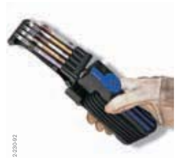
Measuring with the Dräger Simultaneous Test-Set
