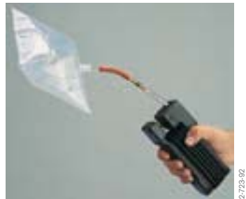
Respiratory CO Test measurement
