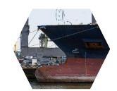
The bulb modifies the way the water flows around the hull, reducing drag and thus increasing speed, range, fuel efficiency, and stability. A bulbous bow also increases the buoyancy of the forward part and hence reduces the pitching of the ship to a small degree.
