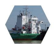
Bridge. The bridge of a ship is the room or platform from which the ship can be commanded. The bridge is manned by an officer of the watch aided usually by an able seaman acting as lookout.
